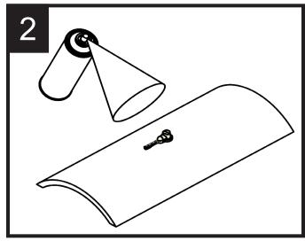
Apply primer to weld and pipe to allow for improved performance.
