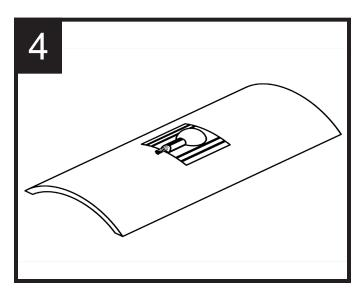
Apply the thermOcap to the pipe by pressing firmly on all edges to insure a proper connection.
