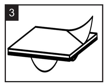
Peal backing from the thermOcap using the attached tag.
