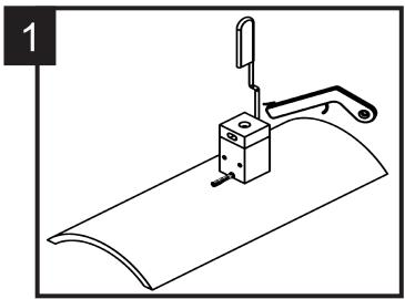
Make your exothermic connection using thermOweld® brand welding products.
